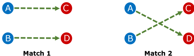
Figure 15: The two possible matches for M = 2 . Blue: nodes from time step t - 1 . Red: nodes from time step t .
