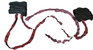
Fig. 3. The point cloud segmented using the PointRend (PR) Object Segment Semantics (OSS) training configuration can be converted to an object mesh for object grasping and manipulation applications.
